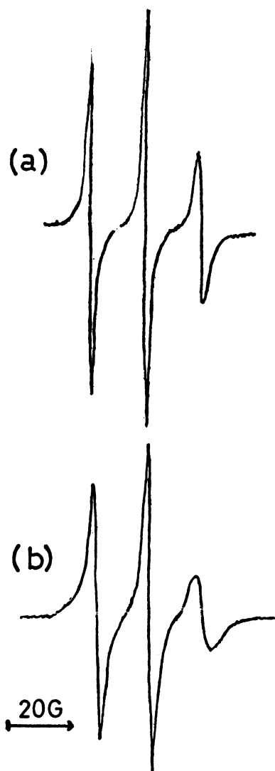
Fig.1. ESR spectra of 1.9 \times 10^{-4} M 12-NS in supercooled solution of NaOH(0.5N). (a), T = -7.35^\circ\text{C} ; (b), T = -20.15^\circ\text{C} .
